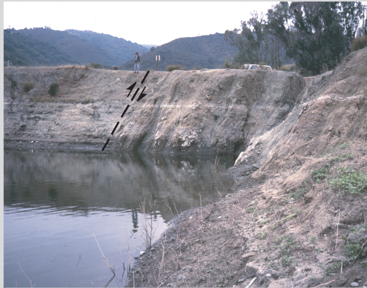
Figure 3B. View N at exposure of the Lexington fault zone east of Lexington dam. Steep dipping 3-4 MA gravels (right) are faulted here against older disrupted bedrock of Mesozoic age (left). Photo location shown on Fig. 3A.
