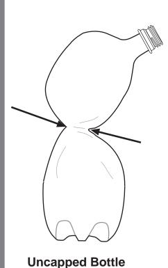
Making a spacesuit bendable is only part of the problem. When an arm or a leg is bent, the bend can reduce the interior volume of the suit and this causes the pressure inside the suit to increase. Consequently, the suit becomes stiffer than before.
