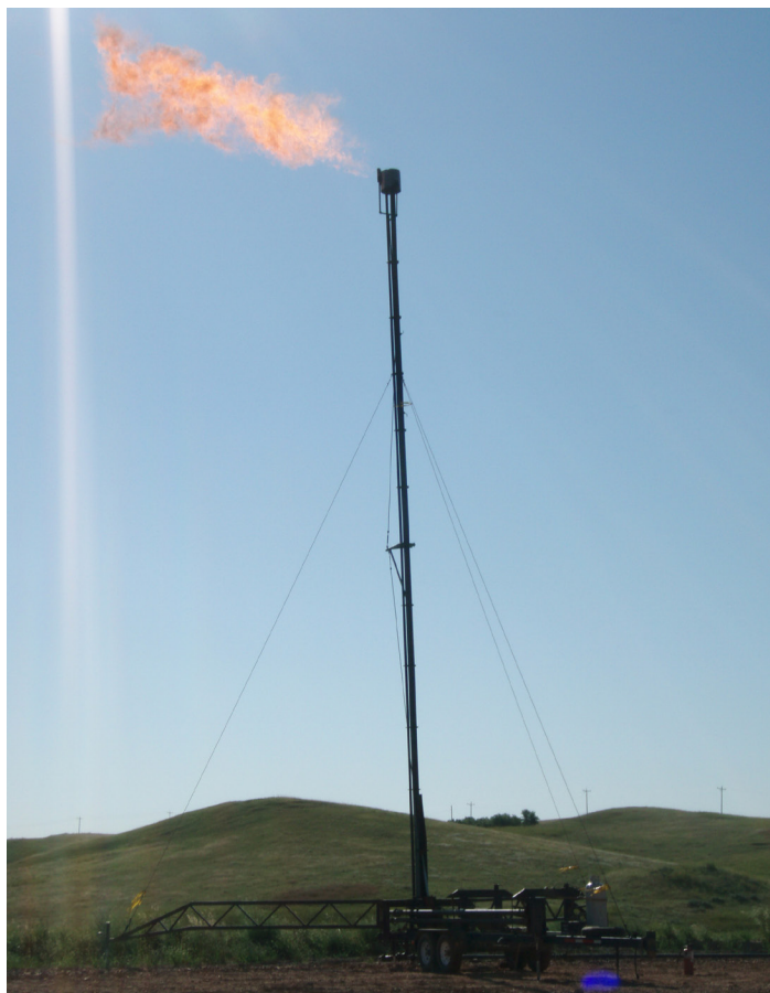
Uncaptured natural gas being flared off in the Bakken oil field, converting the methane to carbon dioxide. Image credit: Wikimedia Commons user Joshua Doubek. 2
