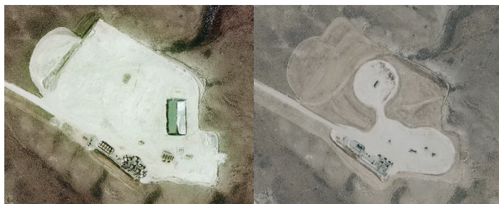
Aerial photos of a well site in the Pinedale Field. Left: Well site during drilling in 2009. Right: Same site in 2015 – the site contains 17 wells, its area has been reduced from 15.3 to 6.04 acres, and the reclaimed 9.26 acres are being revegetated. Image credit: Courtesy of Timothy Zebulske, BLM Pinedale Field Office.
