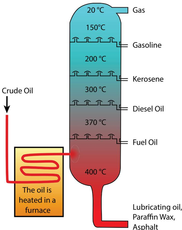
During crude oil distillation, different fuel types condense and are extracted at different temperatures. Image credit: Wikimedia Commons users Psarianos and Theresa Knott.<sup>1</sup>
