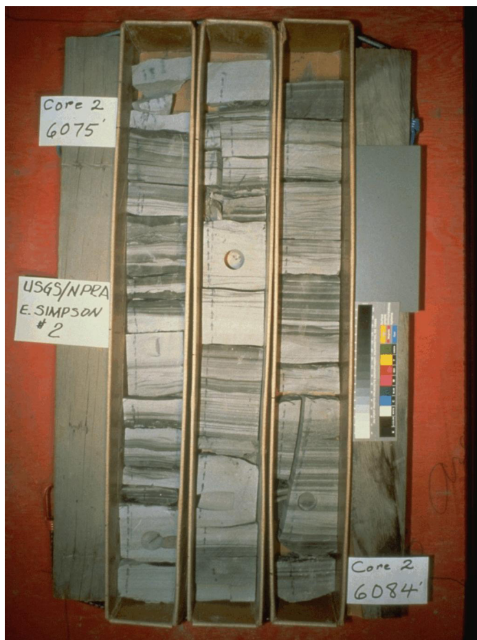
Figure Caption: A box containing 9 feet of 4-inch diameter core from the National Petroleum Reserve, Alaska, showing the fine-scale structure and composition of the rock layers being drilled. Image credit: U.S. Geological Survey. 6
