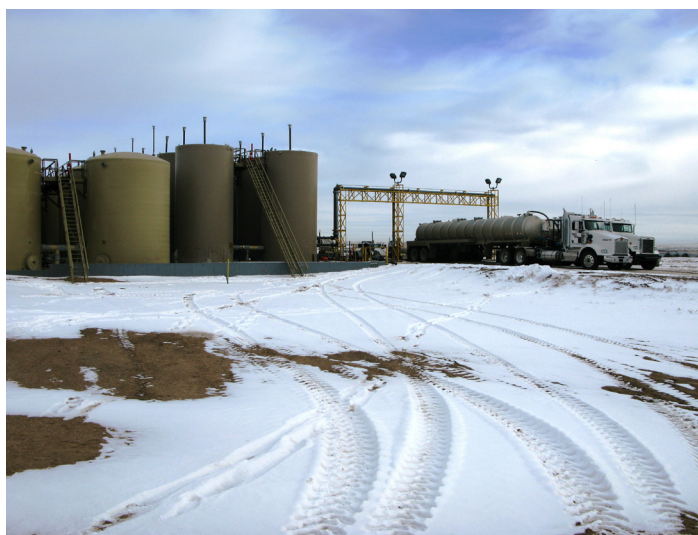
Wastewater is often transported by truck to disposal facilities such as this one near Platteville, Colorado. After some treatment, most wastewater is disposed of deep underground. Image credit: William Ellsworth, USGS. 5
