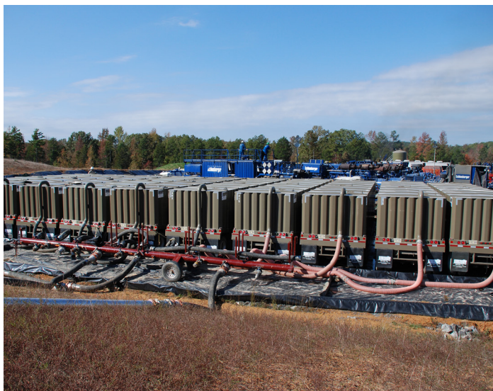
Tanks like these in the Fayetteville Shale area (Arkansas) are commonly used to supply the water required for hydraulic fracturing operations. Image credit: Bill Cunningham, USGS.
