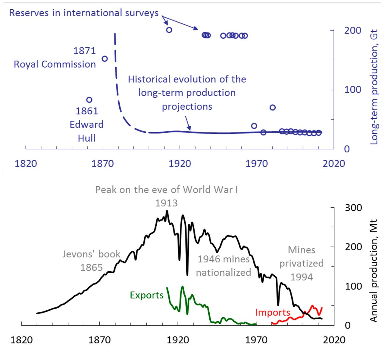
**Figure 7: Change in reserve estimates for UK Coal over time (upper figure) overlaid with actual annual UK coal production in the lower figure (Rutledge, 2013).**
