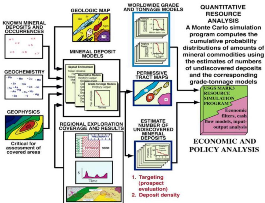
Figure 3: Flow chart illustrating multiple steps of USGS 3-part method for assessing undiscovered mineral resources (from Singer, 2007).
