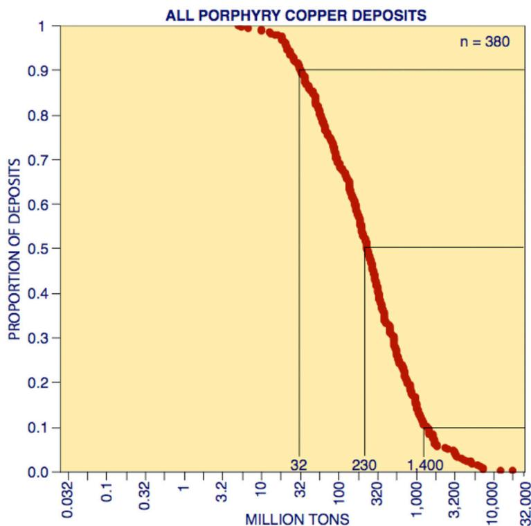
**Figure 5: Tonnage distribution of porphyry Cu deposits. Each point represents a deposit and intercepts are at the 90th, 50th, and 10th percentile (from Singer, 2007).**
