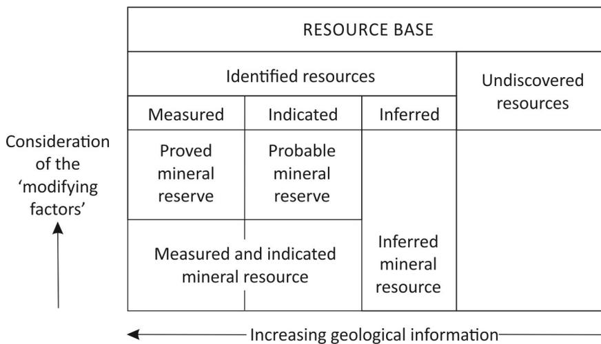
**Figure 1: The relationship between mineral resources and reserves. Mineral reserves generally only represent a tiny fraction of resources. Resource base refers to the total amount of a mineral or metal in the Earth’s crust. \*‘Modifying factors’ include mining, processing, metallurgical, marketing, social, environmental, legal and governmental considerations.**
