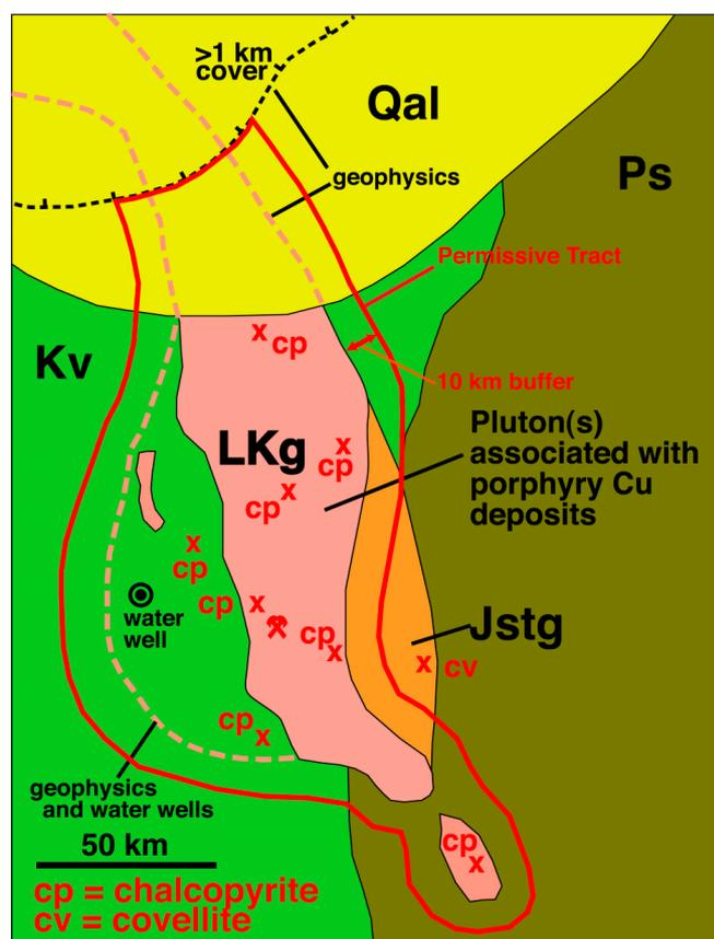
**Figure 4: Boundary of permissive tract is drawn based upon known geology and analogy with the appropriate mineral deposit model (from Singer, 2007).**
