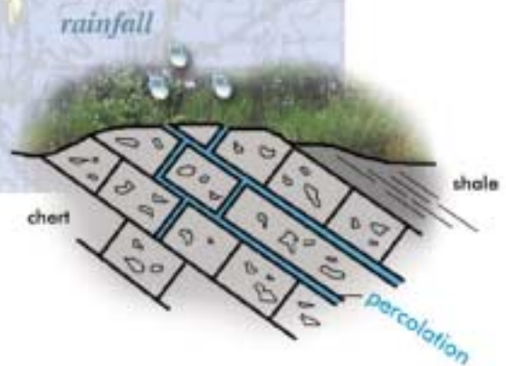
Fig. 4. Where the fractured Fort Payne Chert is exposed, water entering cracks and moving along fractures recharges the aquifer. When this water becomes contaminated, the aquifer and its water resources are at risk.
