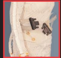
Small, water-filled, plastic tubes laced through the liquid cooling and vent garment keep the astronaut cool inside a spacesuit.
