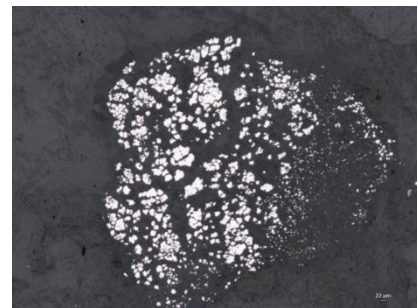
Figure 1: Spheroidal clusters of 'blooming' pyrite grains
