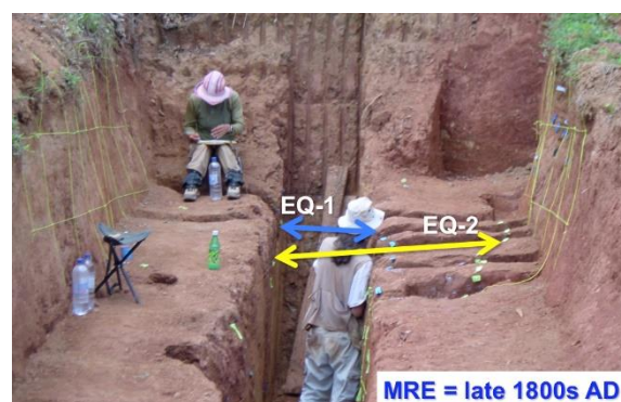
Fig. 2: Hand excavation of small trenches into the eastern bench of Trench T-3 allowed us to define and measure the fault displacement for the most recent (blue flags) and penultimate (yellow flags) events based on the offset of discrete channel margins. The MRE was measured at 0.7 \pm 0.2 m and the penultimate event a cumulative 1.4 \pm 0.3 m. The \sim 500 year third event was displaced beyond the 2 m exposure afforded by the bench.
