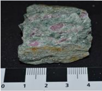
Figure 2. Coarse-grained actinolite schist with subhedral rubies to 20mm.
