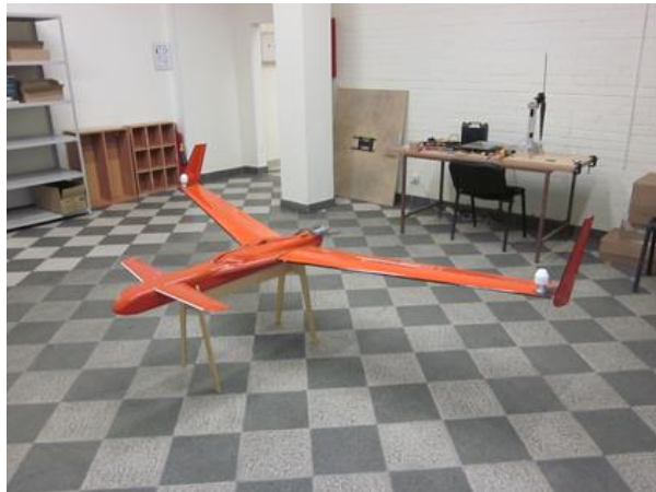
Figure 1: Non-magnetic unmanned aerial platform
