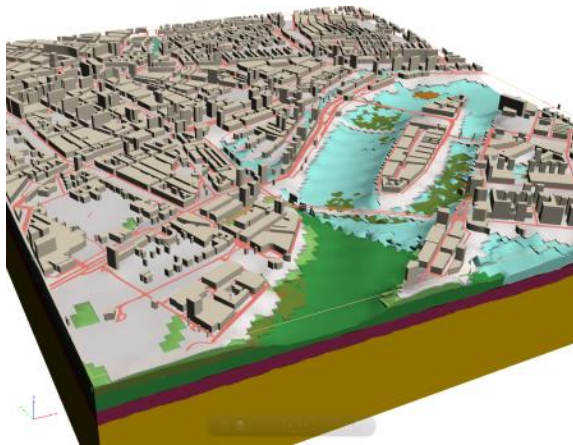
Figure 1: Geological voxel model of Rotterdam
