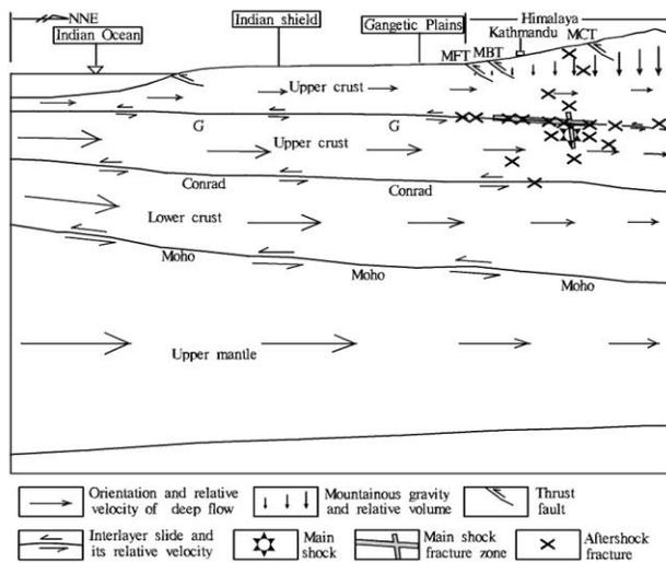
*Figure 1: Schematic diagram of the geodynamic framework within the lithosphere and its control over the earthquakes around the earthquake-stricken region of Nepal. MFT: main frontal thrust; MBT: main boundary thrust; MCT: main central thrust. G: top face of the crystalline basement*
