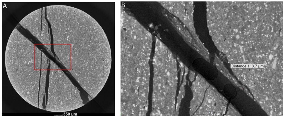
*Figure 1: X-ray CT investigation of Opalinus Clay, sandy facies A) shear failure (diagonal) and diking (vertical) and B) gouge zone in the field of shear failure.*
