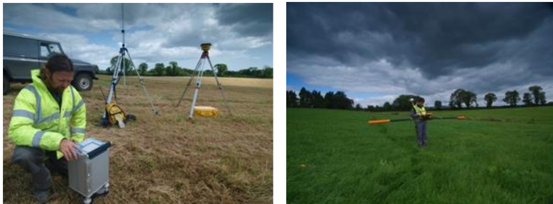
Figure 1: Typical surface geophysical methods; (Left) Microgravity. (Right): EM31 Survey
