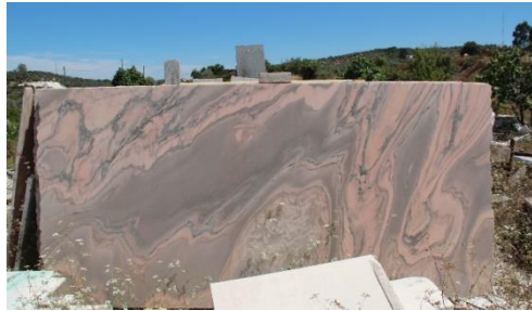
Figure 1: Slab sawed perpendicular to principal metamorphic orientation showing two fold interference patterns.
