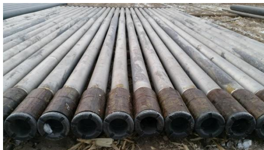
Figure 1: Aluminum alloy drill pipe with steel joints
