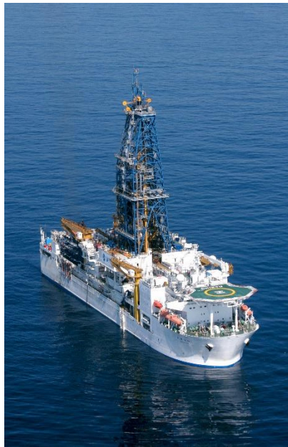
Figure 1: D/V Chikyu . Riser equipped scientific ocean drilling vessel.
