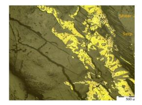
Figure 1: Reflected light microscopy of a) Sample JDJ-12A from T1 with replacement of sulphides by secondary silicates; b) Sample JDJ-15 from T1 illustrating the partial remobilisation of chalcopyrite and pyrrhotite along a vein and possible shear zone.
