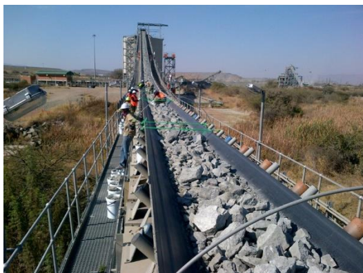
Figure 1: Collecting the 500kg bulk sample used for the test work from the temporarily stopped conveyor belt.
