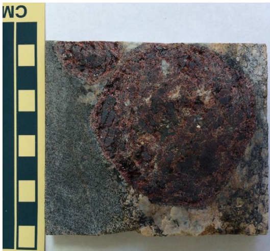
Figure 1: Garnet porphyroblast in leucosome of metapelite from Cauchon Lake, Pikwitonei Granulite Domain, Canada
