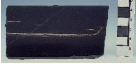
Figure 1: Chalcocite and bornite epigenetic vein structures in black Cu-bearing shale (scale bar in centimeters), Rudna Mine .
