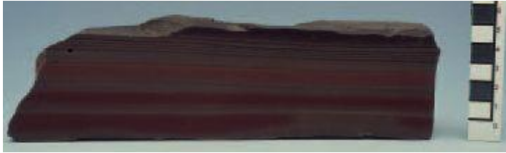
Figure 1: Chalcocite and bornite epigenetic vein structures in black Cu-bearing shale (scale bar in centimeters), Rudna Mine .
