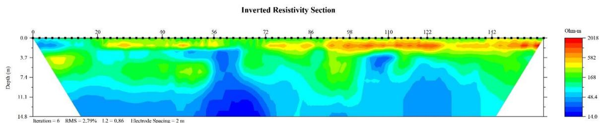
*Figure 1: Two dimensional electrical resistivity model for the study area. The sea is at 0 m.*
