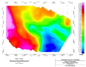
Gravity Bouguer anomaly map (figure.1) reveals lows in the south eastern end of the surveyed area with a gradual increase towards the western part which could be associated with a boundary between the Eendoorn suite and Narries semi-Pelitic granulites. Response from the radiometric and Landsat-8 data was largely interpreted to be associated with the water drainage patterns and topography within certain parts showing lineaments trending from northwest to southeast.
