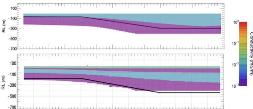
Figure 1. Inversions of a 25° dipping conductive wedge of 100Ωm, (top) in a resistive basement of 1000Ωm (bottom) 100m below a 50Ωm, 40m thick regolith, in a 1000Ωm resistive basement.
