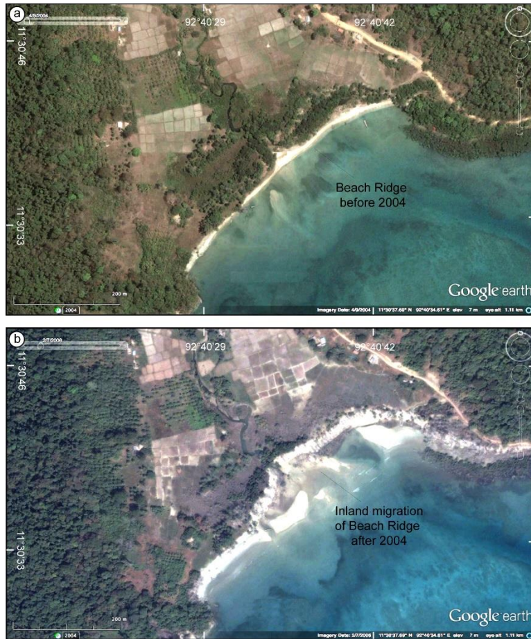
Figure 1: (a) Google earth image showing beach ridge and a back marsh before 2004 Sumatra-Andaman earthquake, (b) Subsidence and inland migration of beach ridge. Formation of back marsh further inland.
