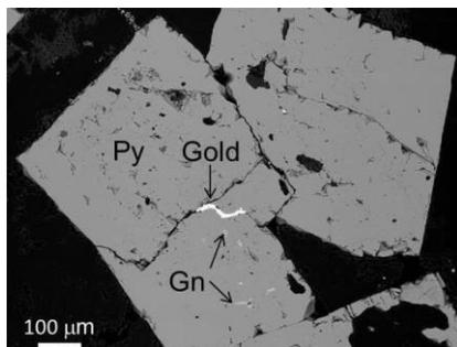
Micron-size gold grains were detected within pyrite and between pyrite crystal boundaries (Fig.1). Assay data of drill core samples indicate gold grades in mineralized phyllites and schists ranging from 0.02 to 0.54 ppm, and from 0.2 to 3.8 ppm, respectively. Elevated Au values are generally found in the hydraulic brecciated schist. There is no clear relationship between gold and base metal content, however samples with high gold values tend to contain low copper, lead and zinc.
