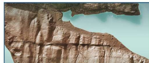
In this composite lidar/photo image, the Toe Jam Hill fault scarp (a strand of the Seattle fault zone) is clearly visible in the landscape on Bainbridge Island in Washington. When viewing only the aerial photo, the fault scarp is not visible due to tree cover and infrastructure on the island. Credit: The all-Geo, with rights from Department of Natural Resources.
