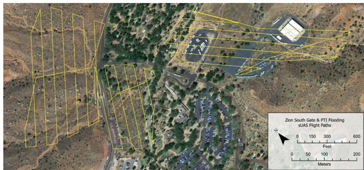
Drone flight paths are typically planned prior to takeoff to ensure that they can collect the needed data. Here, the drone flight paths (yellow lines) used to collect imagery data for structure from motion (SfM) modeling and lidar data comparison at Zion National Park are displayed. Credit: Utah Geological Survey
