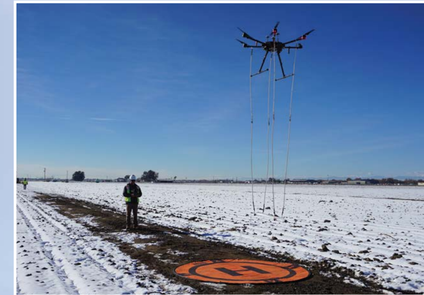
A magnetic survey is conducted in Colorado using a UAS-enabled magnetometer to locate buried orphaned wells and buried pipelines. Credit: Nathan Campbell, EDCON-PRJ. Jack Davis, Juniper Unmanned
