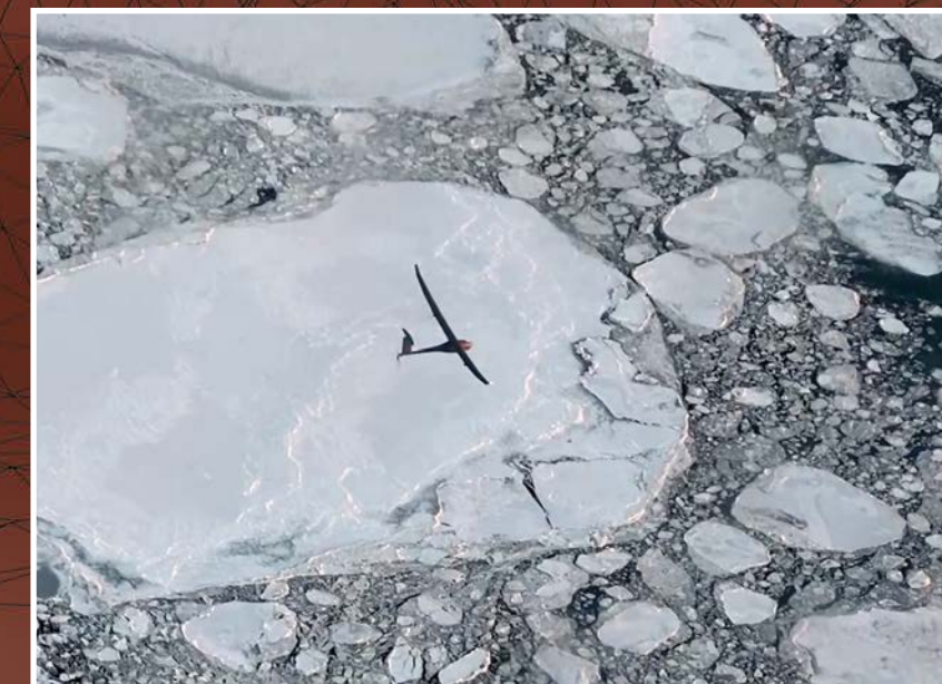
A fixed-wing drone named Vanilla , flies over sea ice in the Arctic to survey snow depths under NASA ICESat-2 ground tracks. Credit: Toby Woods, 70 North LLC
