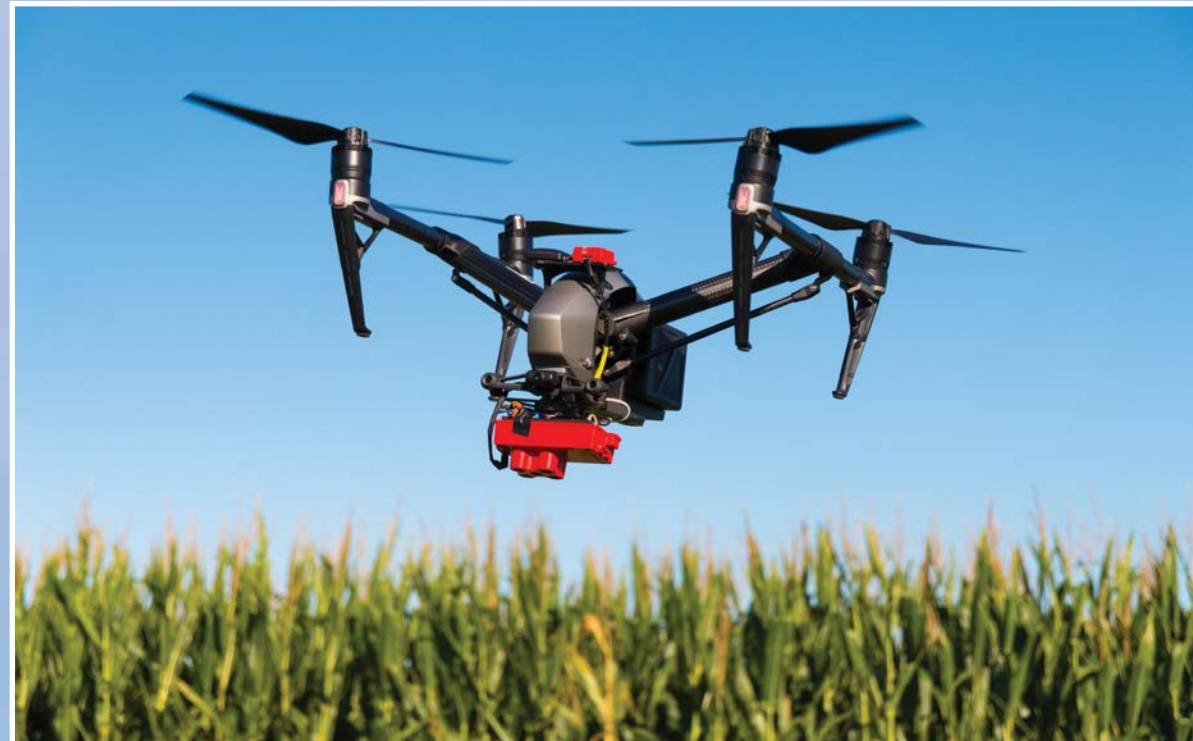
A drone equipped with a multispectral sensor flies over a Nebraska cornfield. It is capturing images to generate a vegetation index map. Credit: Laura Thompson, UNL
