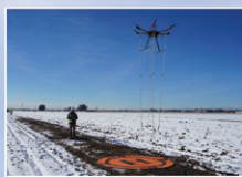
A magnetic survey is conducted in Colorado using a UAS-enabled magnetometer to locate buried orphaned wells and buried pipelines. Credit: Nathan Campbell, EDCON-PRJ, Jack Davis, Juniper Unmanned
