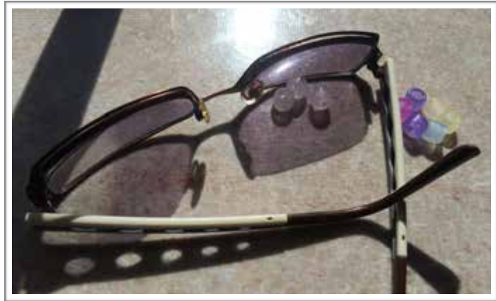
UV beads in a sunny (but closed) window. Note that the beads shaded by the lenses are uncolored - these glasses provide UV protection.
