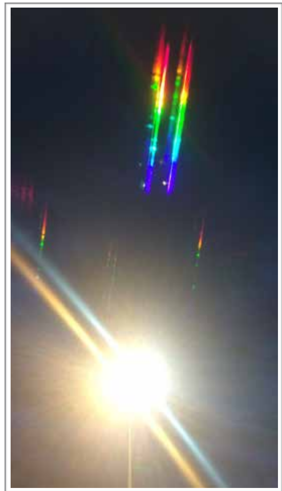
Two different types of bulbs on the same post. Note that the pattern of bright spots in the spectra are slightly different.
