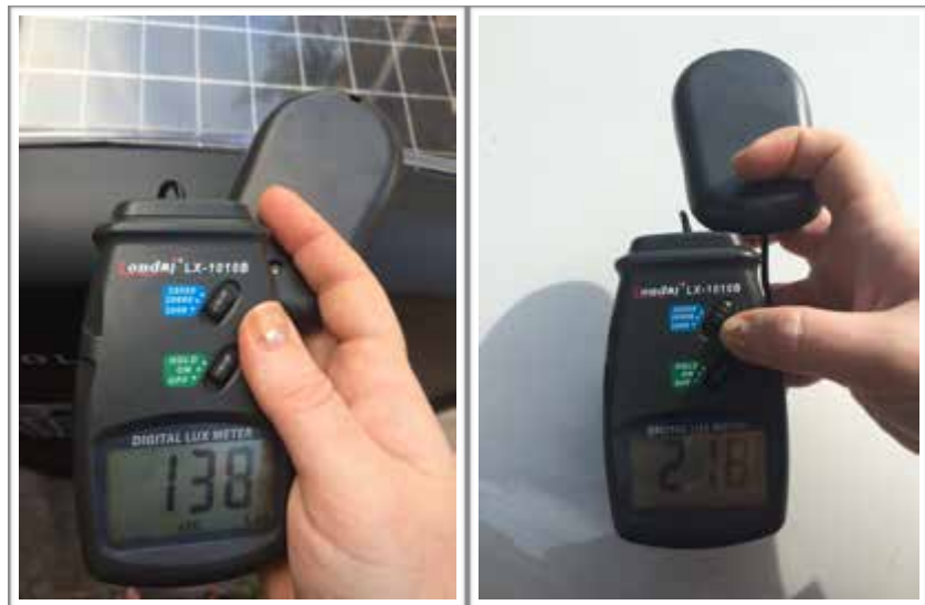
Left: measuring the reflectance off a black plastic bin (1380 lx). Right: measuring reflectance of a white car (21800 lx). Note readings are at different scales and readings need to be multiplied by 10 (left) and 100 (right).
