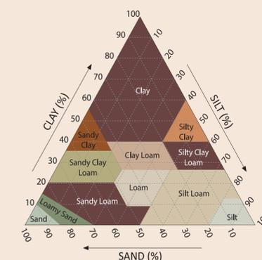
This diagram is used to identify soils by the relative amounts of silt, clay, and sand they contain.
