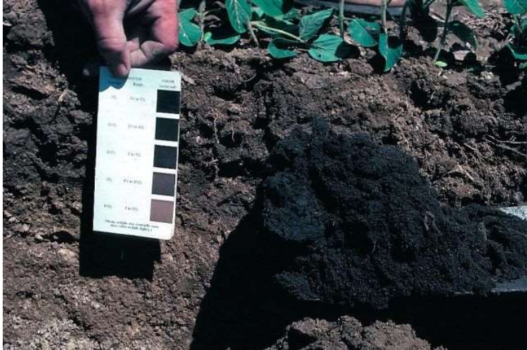
Figure 1. A soil profile being compared to a Munsell color chart, which can help determine soil properties. Credit: Betts.
