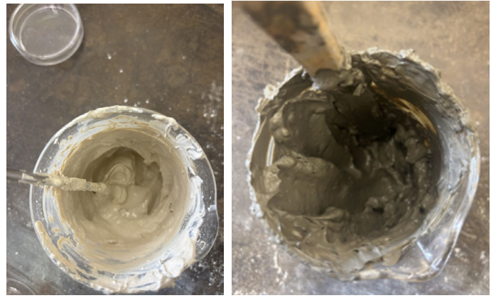
Clay mineral kaolinite sample (left) and montmorillonite sample (right) in a thick slurry with no standing water in a 200 ml beaker.
