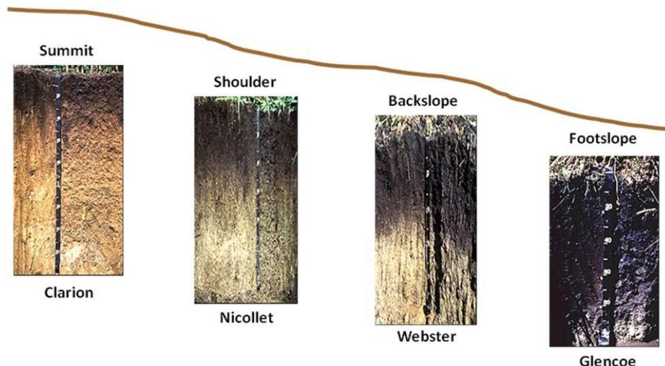
Soil profiles reveal distinct layers, or horizons, that reflect how soils form and change. Notice the gradient of soil color from oxidizing conditions at the summit (red/brown subsurface colors) to reducing conditions at the toe slope (gray subsurface colors) for representative soil profiles of the Clarion-Nicollet-Webster catena.
