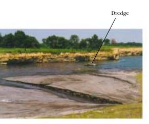
Fig. 32. The dredge in this slurry pond is removing material from which fine particles of coal will be separated and collected (remined) for use.
