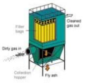
Fig. 42. Diagrams of fabric filters and electrostatic precipitators (ESPs), which are used to capture particulate matter.
