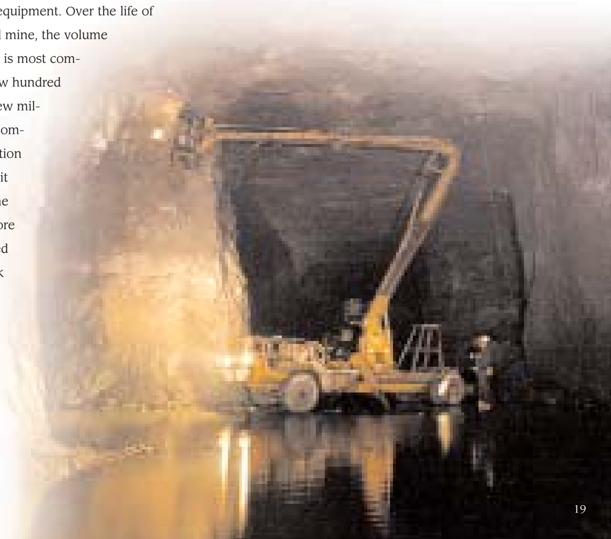
Fig. 5. Large equipment used in underground mining includes scalers that remove loose materials left on the walls and roof after blasting.
