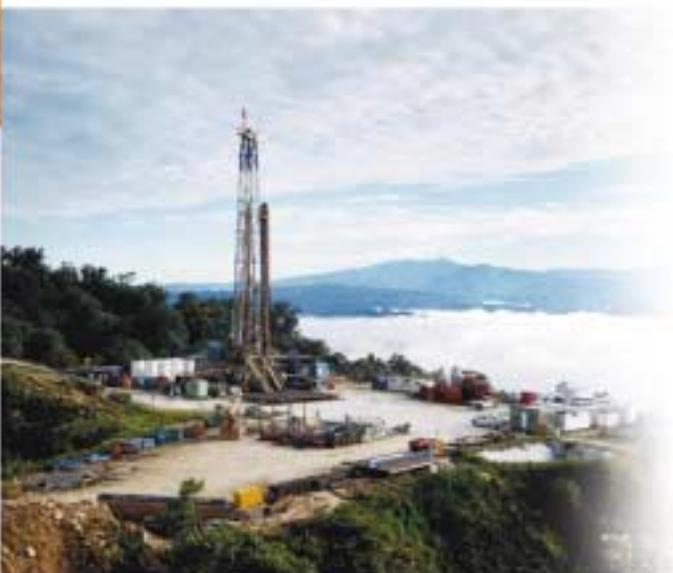
Fig. 15. This drill rig in Papua New Guinea was lifted into place in sections by helicopter, thus minimizing the need for extensive jungle clearing and road building. The four-wheel trucks shown here came up narrow mountain roads that could not be used by larger vehicles.
