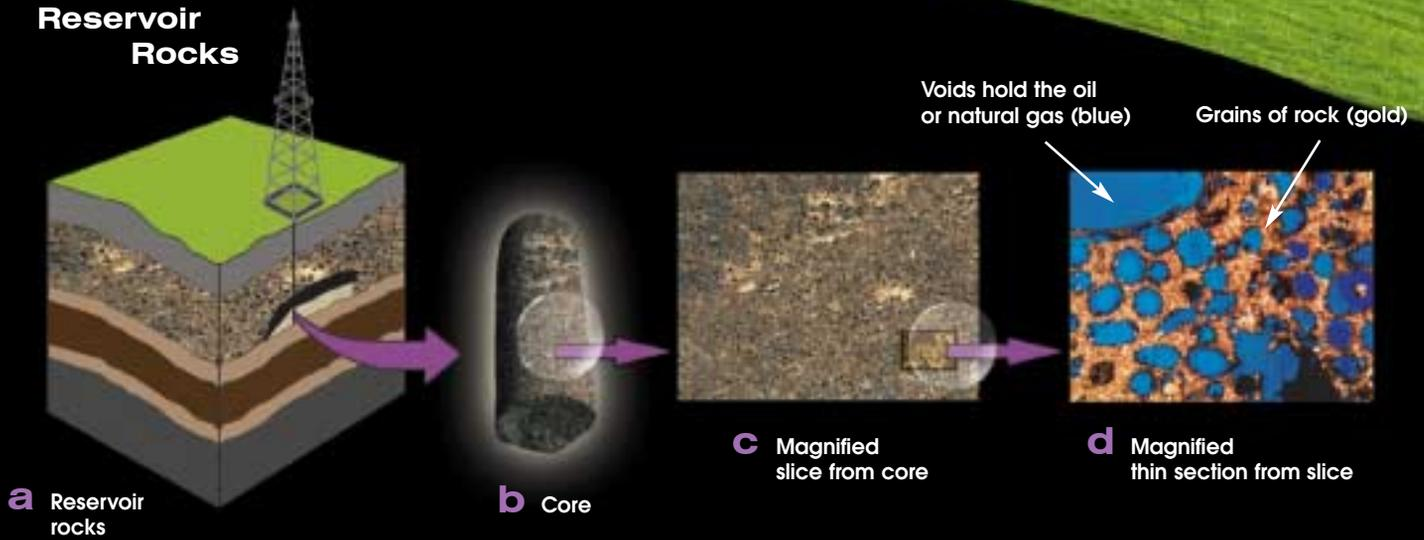
Fig.9. (a) Limestone and sandstone are sometimes porous enough to become Earth's underground reservoirs for oil and natural gas. (b) A rock core was taken from a depth of a few thousand feet. (c) A small piece cut from the core was ground so thin (to the thickness of a piece of paper) that light passes through it. (d) Magnification of this "thin section" exposes the tiny spaces (blue) where oil and gas are stored among the grains of rock (gold).
