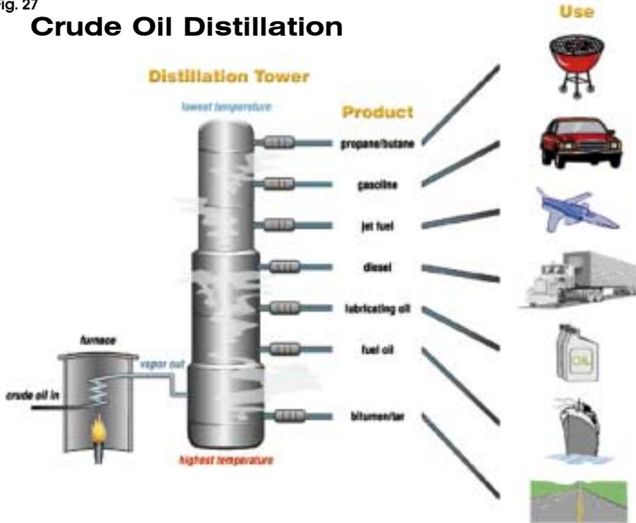
Fig 27. Distillation is a key process in refineries and allows a complex mixture of hydrocarbons to be separated into many types of consumer products.
