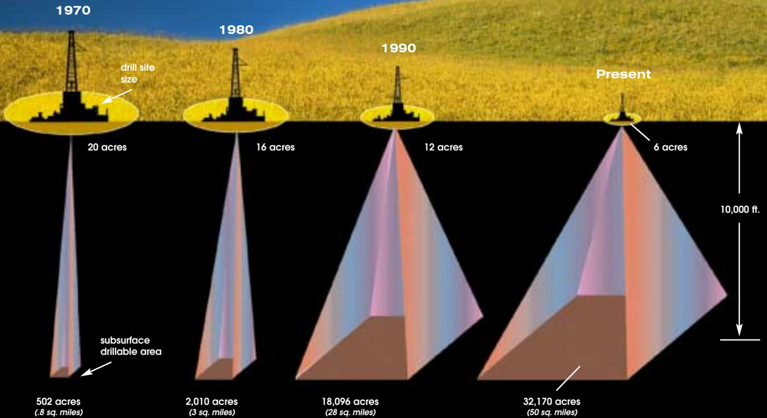
Fig. 25. Major improvements in drilling technology over the last 30 years have resulted in much smaller drill sites.
