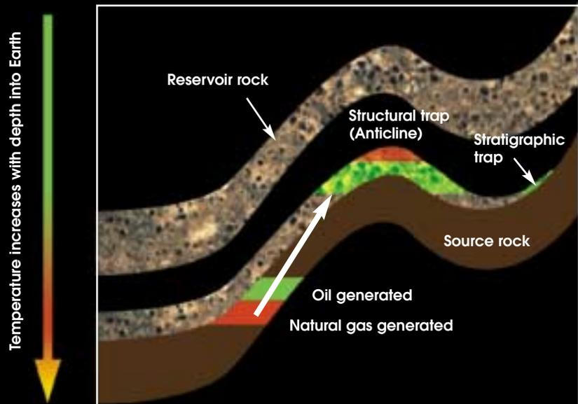
reservoir rock to hold petroleum topped by an impermeable layer that serves as a seal and barrier to further migration creates a geologic feature called a **trap** (Fig. 10). Because subsurface traps are primary sources of crude oil and natural gas accumulations, they are the ultimate target of petroleum exploration programs.
