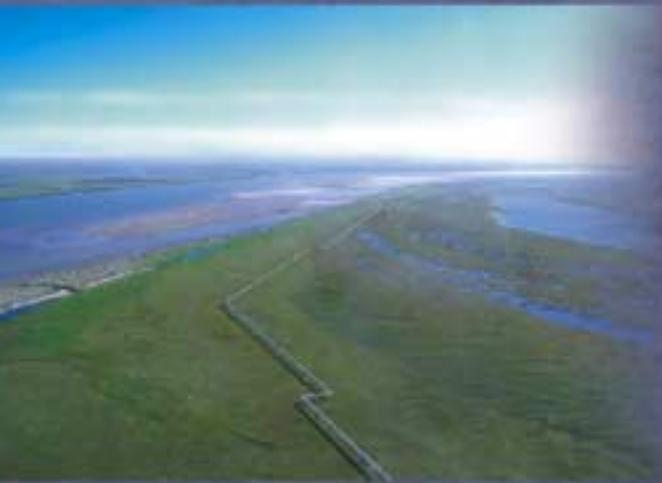
*The pipelines needed to transport oil from Alpine were placed 100 feet below the Colville River eliminating the need for a bridge.*
