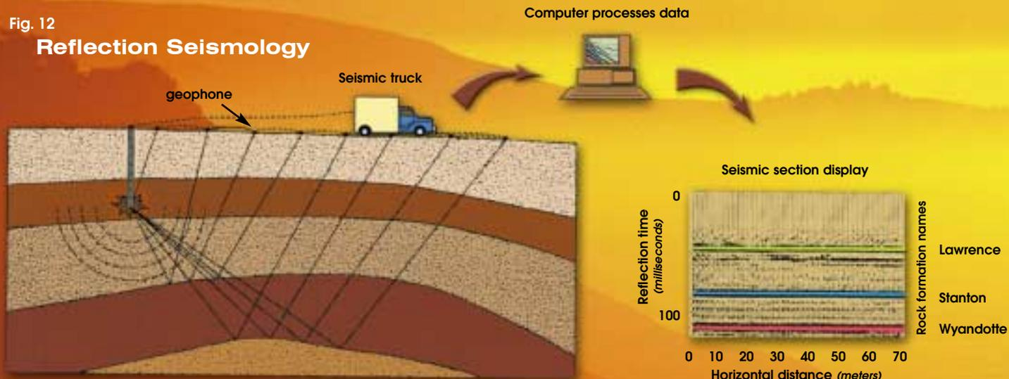
Fig. 12. Sound waves from an energy source are reflected upwards when a change in rock properties is encountered. The major components of a seismic system include a source of energy, sensors (geophones) laid on the ground to record sound waves, and a computer to process signals.
