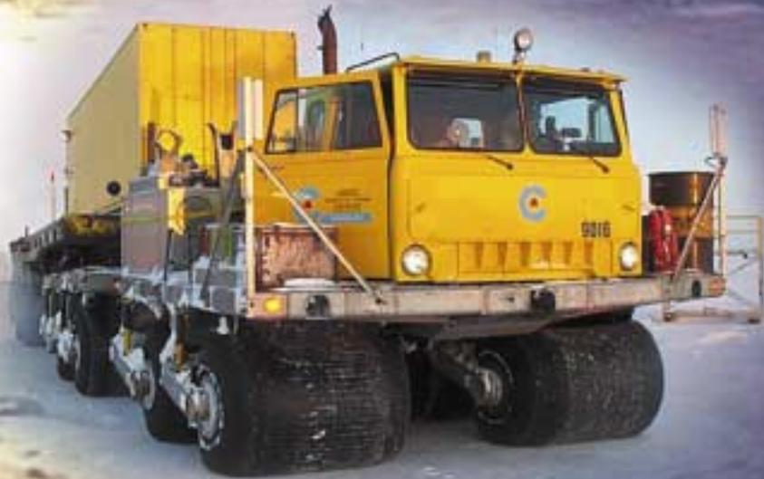
The large low-pressure tires on rolligons prevent damage to the permafrost. Alpine is the first production facility on the North Slope to depend entirely on temporary ice roads to provide access. As summer approaches, the ice roads melt away leaving the tundra undisturbed. Only aircraft service the Alpine production facility during the summer.
