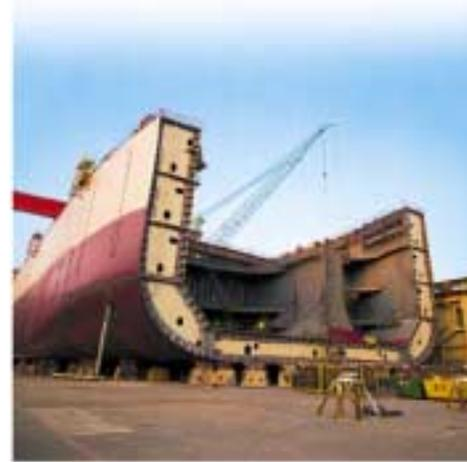
Fig. 34. The Oil Pollution Act requires that by 2015 tankers operating in U.S. waters have double-hulls. Many double-hull tankers are already in service, and their value in terms of environmental protection has already been demonstrated.
