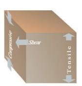
Fig.16. *Soil tensile, compressive, and sliding (shear) strengths.*
