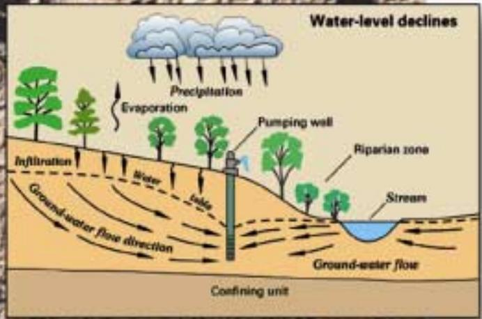
Fig. 25. Pumping removes groundwater from storage. This can intercept groundwater that would normally discharge to the stream and divert stream water to the well.
