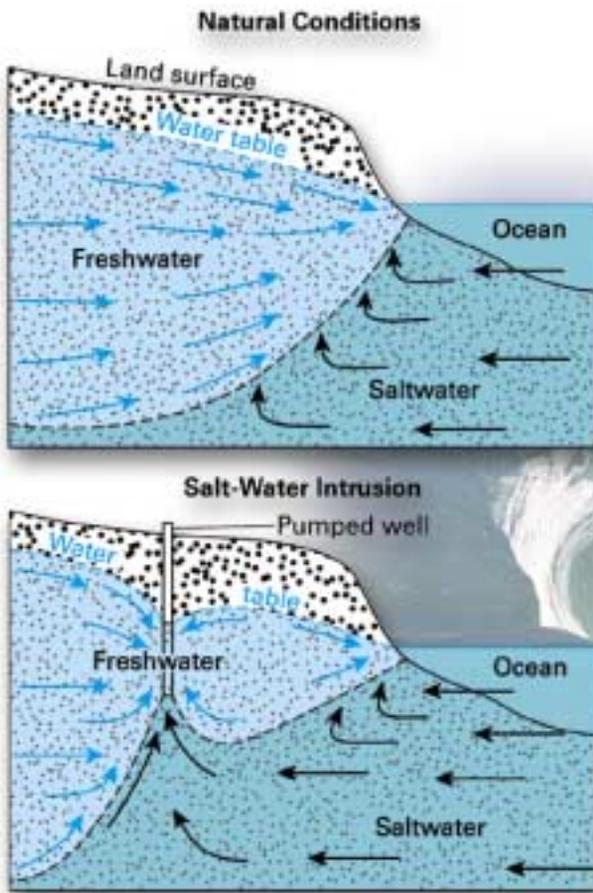
Fig. 28. Intensive groundwater pumping can cause salt-water intrusion in coastal aquifers.
