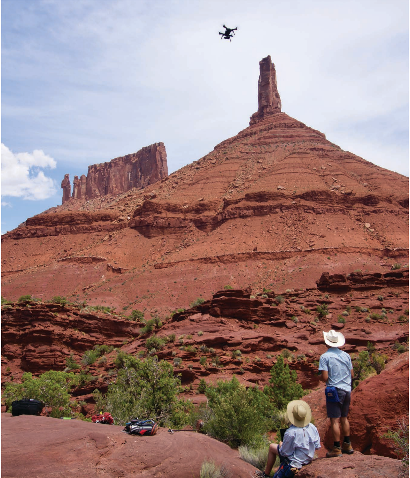
Nicholas Perez for AGI's 2017 Life as a Geoscientist contest Clyde Findlay, Ph.D. student, and Keller Herrin, undergraduate research assistant, from Texas A&M University, conduct a drone survey near Castleton Tower, Utah. They will use the series of aerial images to create a 3D outcrop model, and combine the results with field measurements to investigate stratigraphic questions about the upper Paleozoic Cutler Group.
