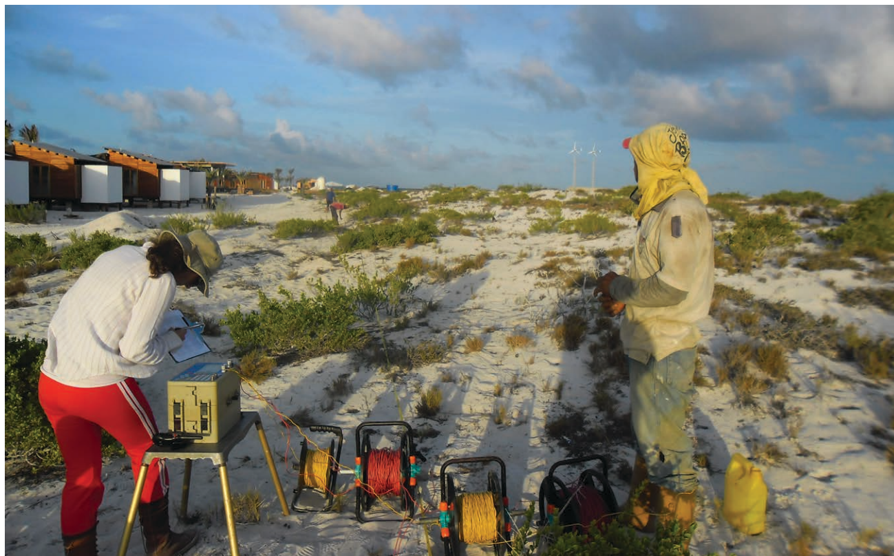
Carianna Herrera for AGI's 2017 Life as a Geoscientist contest La Tortuga Island, Venezuela. Geophysical acquisition with conventional geoelectric methods for groundwater exploration along the runway of the island.
