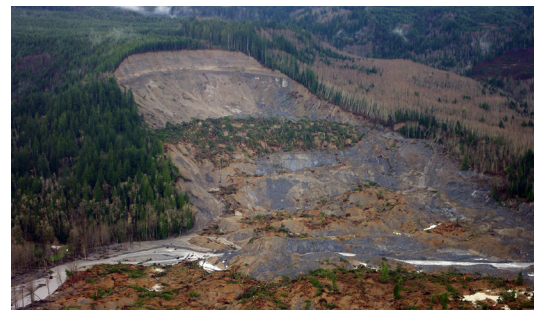
The 2014 Oso landslide moved an estimated 270 million ft 3 of rocks, dirt, trees, and other debris down the slope. The direct costs for repair are greater than $80 million.
