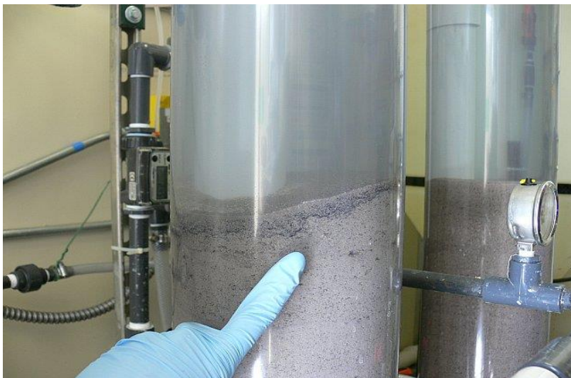
Coal fines accumulating in the modified zeolite filtration medium.
