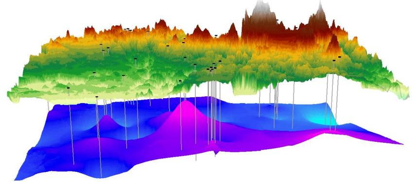
Generalized bedrock projection using ~42 data points.
